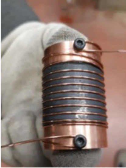
Figure 1. VAMAS barrel ready for the heat treatment.
