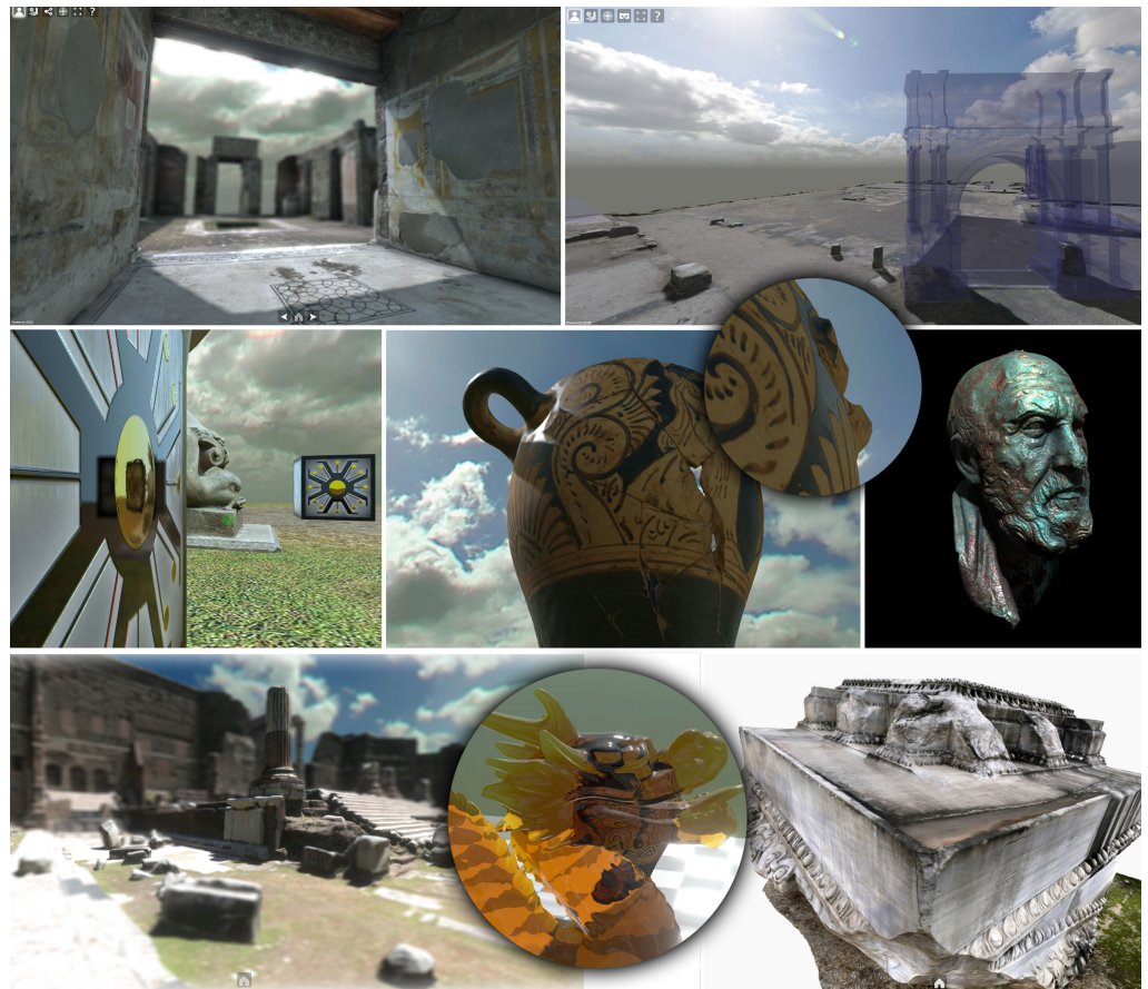
Figure 8. A few captures from interactive 3D scenes in ATON. Top row: real-time shadows and advanced effects (bloom, ambient occlusion); Middle row: multiple light-probes system and PBR materials; Bottom row: depth-of-field effects, real-time volumetric refraction and absorption (Khronos glTF extension) and multi-resolution dataset (Cesium 3D Tiles)
