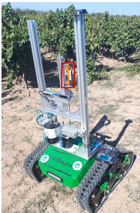
Fig. 2. The farmer robot, used for data acquisition, equipped with a side-view Intel RealSense D435 camera (red framed) and a GPS sensor. Additional sensors shown in the picture, such as a 2D lidar and frontal cameras, are not used in this work.
