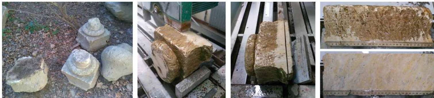
Fig. 3 Sample altered by external exposure: in situ location (left), laboratory cutting steps (center), specimens obtained for testing (right).
