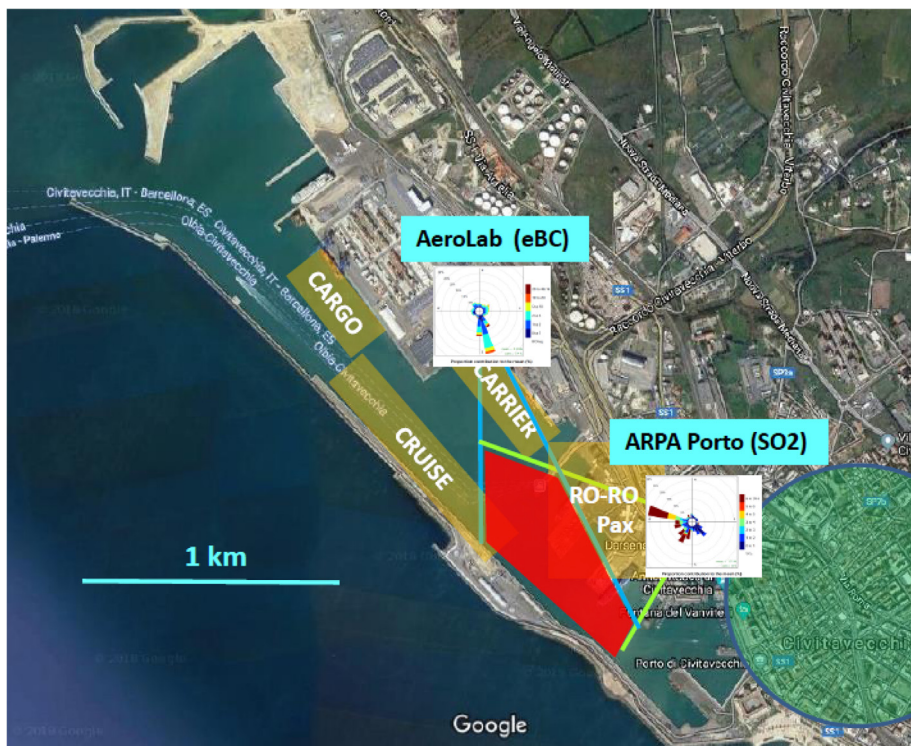
Fig. 6. Triangulation between origins of maximum eBC sources (as measured by the AEROLAB at Pier 24), and maximum SO 2 sources (as measured at Arpa Porto), during the April 2016 campaign. The Civitavecchia city center is indicated by the blue circle at the bottom right end of the figure. (For interpretation of the references to color in this figure legend, the reader is referred to the web version of this article.)
