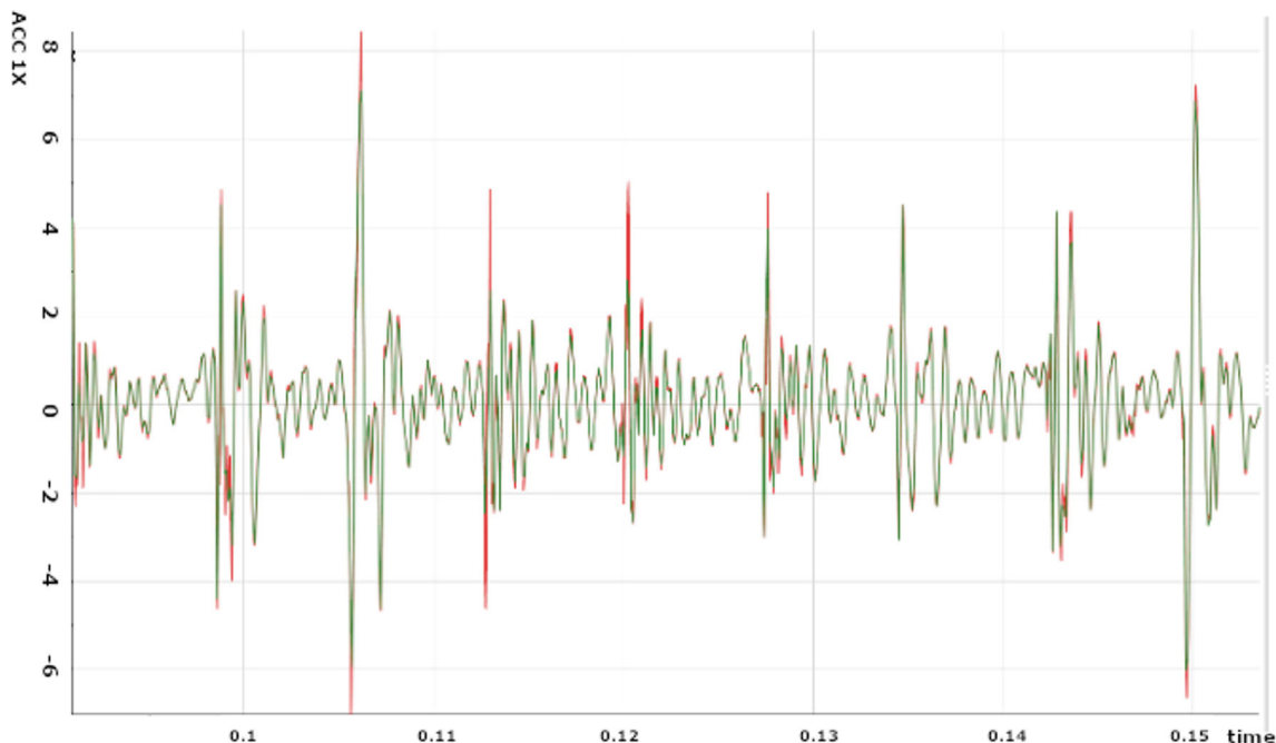
Fig. 4 Superposition of Acc1X of nominal test, original (red) and resampled 10,000 Hz (green)
