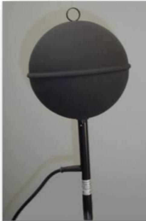
**Figura 36: globotermometro**
