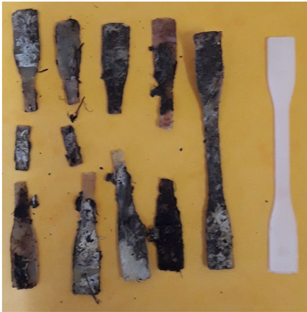
Fig. 11 Intermediate visual inspection on neat PBSA specimens after 20 days of industrial composting disintegration test occurred in Composter: on the right side the starting dog-bone specimens
