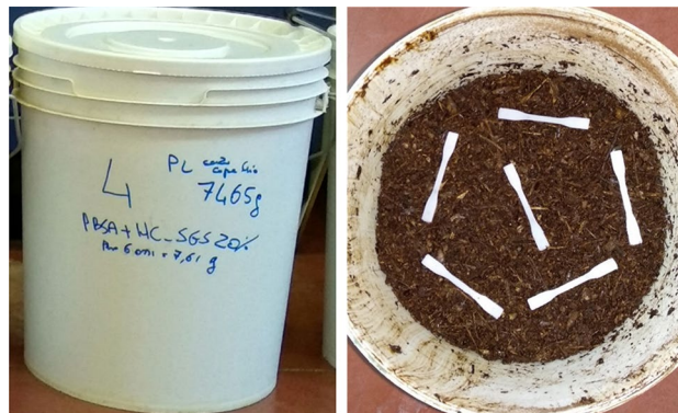
Fig. 3 Dog-bone specimens buried into compost kept indoor at room temperature, undergoing the mesophilic curing phase for the home composting disintegration test
