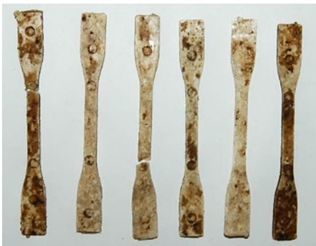
Fig. 14 Specimens of PBSA/HCa 5% after 259 days of home composting disintegration test
