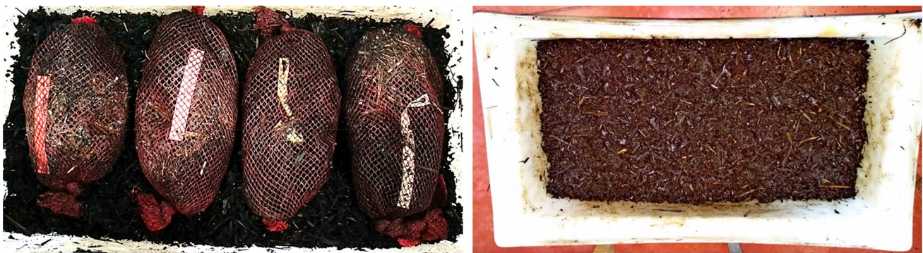
Fig. 10 Different specimens in separated PE net bags and buried into compost at room temperature (second curing phase, from 45 to 84th days)
