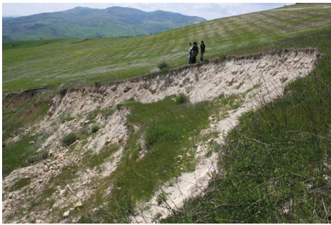
Figure 5. Crown area of one of the sources of the Alberona mudslide, showing a clear rotational character.
