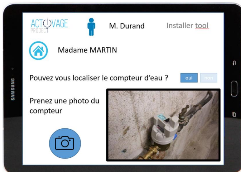
Figure 78. Installer tool mock up: discovering the existing asset, in this case the water counter and valve
