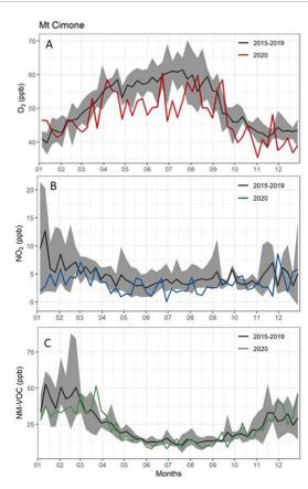
**Figure 3.** Weekly average  $O_3$  (A),  $NO_2$  (B), and NM-VOCs (C) values at CMN, in 2020 (colored lines). The gray area denotes the envelope of single years from 2015 to 2019. The black line indicates the average value over 2015–2019.
