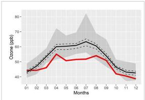
**Figure 1.** Monthly average  $O_3$  at CMN from 1996 to 2020 (the thick black line represents the monthly mean values from 1996 to 2019, the red line indicates 2020 data, the dashed lines represent the 95% confidence level, and the gray area represents the range of monthly mean values from 1996 to 2019).
