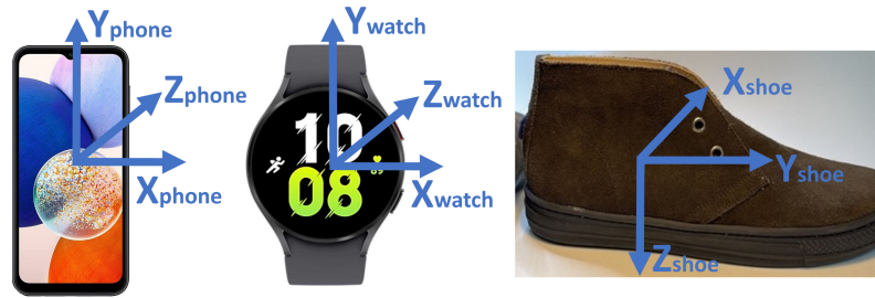
FIGURE 1: TOLIFE wearable set: smartphone (left), smartwatch (center), smart-shoe (right). Local reference frames associated with the inertial sensors are reported. The left shoe reference is defined symmetrically to the right shoe.
