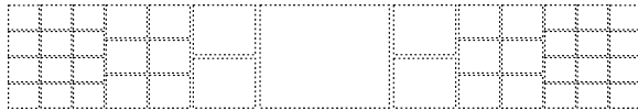
Figure 4: Another example of layout of slots (as in Fig ??), this time for a PileBar with a rectangular shape.
