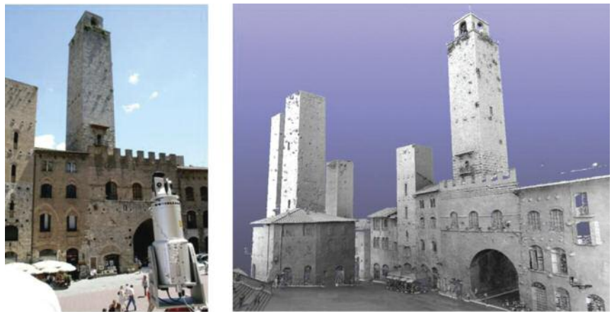
Figure 1: Acquisition of the tower's geometry by means of a TOF laser scanner (on the left), 3D digital model of the Rognosa tower and the Cathedral Square (on the right).
