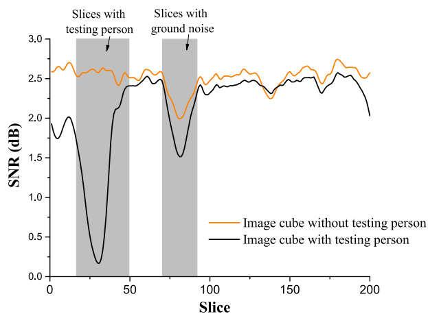
FIGURE 7. Signal-noise ratio of an image cube with testing person and one without testing person. Testing person is in slices 20 to slice 50, while ground noise exists in slice 70 to slice 90.
