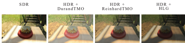
Figure 6: An example of the “Jelly2.0” scene showing the different types of input images used in our work: 0-stop SDR images, ReinhardTMO images, DurandTMO images, and HLG HDR images.
