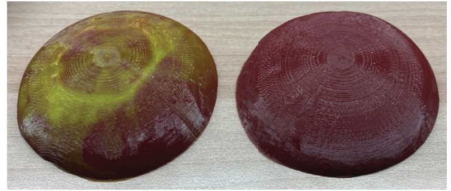
Figure 2: Liver phantoms: On the left is the fatty liver phantom, characterized by a yellowish color. On the right, there is the healthy liver phantom, characterized by a reddish-brown color.
