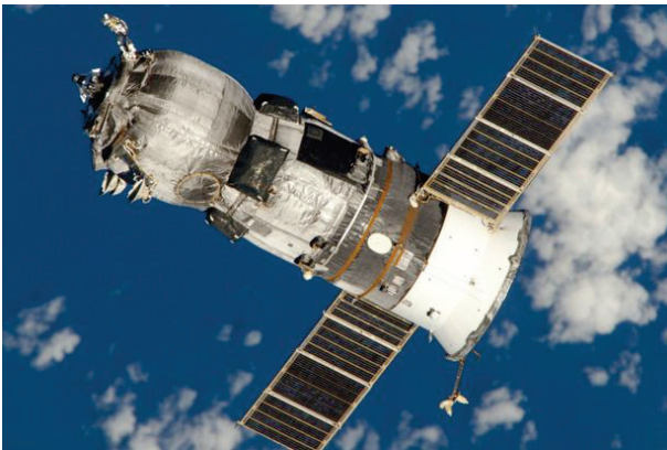
Figure 2. A Progress-M cargo vessel, with a length of 7.23 m, a maximum diameter of 2.72 m and a maximum solar panels span of 10.6 m (courtesy of NASA)
