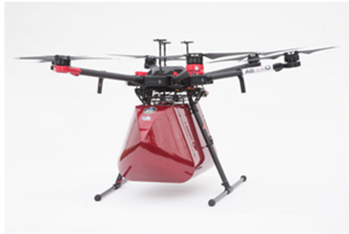
Figure 2. The drone-based delivery system equipped with the smart capsule.
