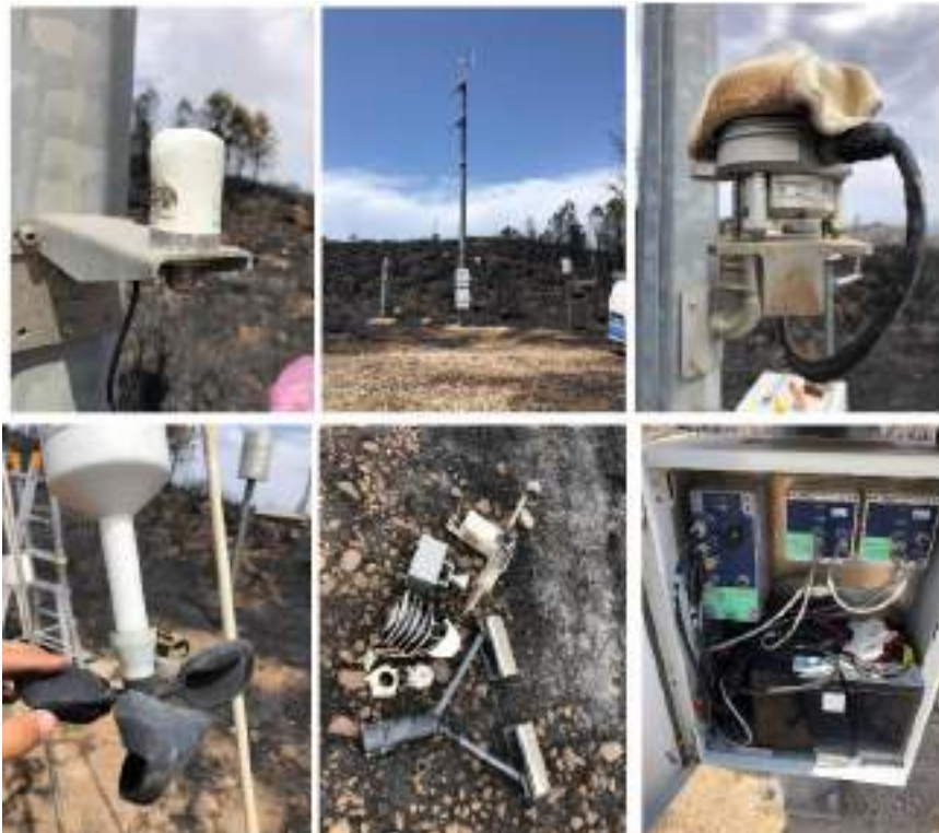
Figure 50 – Temperature and relative humidity, and wind intensity measured in the Badde Urbara (1,033m a.s.l.) weather station. The dotted line highlights when data of temperatures and humidity are not reliable as they refer to the period following the passage of the fire. The third image is evidence of the damage to the weather station caused by the wildfire.
