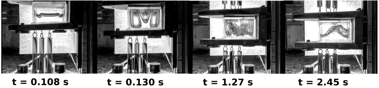
FIG. 2: Experimental snapshots of the SDOF vertical sloshing water experiments carried out in [15] for 10 g and 50 % filling level.
