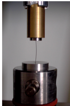
FIGURE 3. The supporting beams of the dynamometer equipment for the buckling measurement
