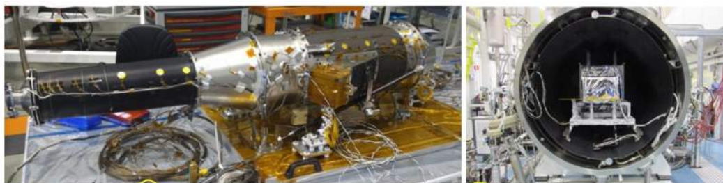
Fig. 25. Metis structural thermal model prepared for the vacuum thermal-balance test with temperature sensors installed inside and on the external surface ( left ). Metis structural thermal model inside the thermal-vacuum chamber endowed with Sun simulator, at ESTEC/ESA ( right ).
