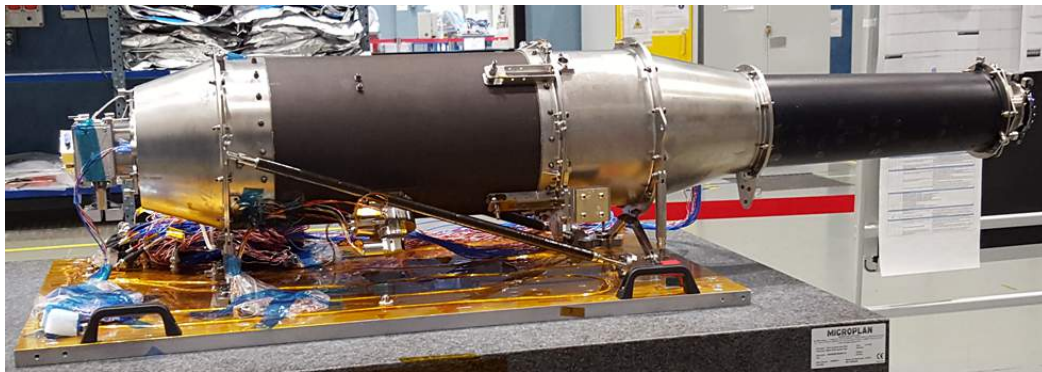
Fig. 23. Structural qualification model of the telescope prepared for the sine and random vibration tests.
