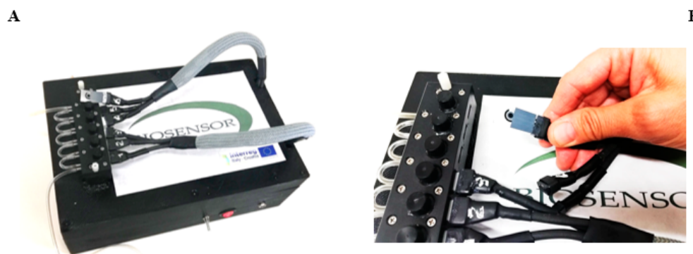
Figure 1. (A) Algal cytosensor prototype equipped with six measurement cells, fluidics, and the opto-electrochemical set-up, (B) Screen-printed electrode ready for the insertion into the measurement cell. Dimensions of the instrument: L28.5 \times I19 \times H10 cm.
