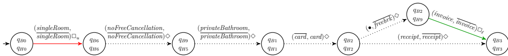
Figure 6: Orchestration of composition BusinessClient \otimes Hotel of the two automata in Figures 2 and 3 for the canonical product P4859
