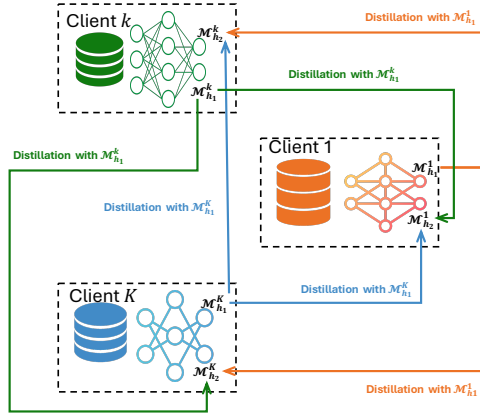
Fig. 2: KD-based decentralized network consisting of K clients, where distillation is performed using soft labels for effective knowledge transfer. In this setting, the first head of each client is communicated to the neighboring clients.
