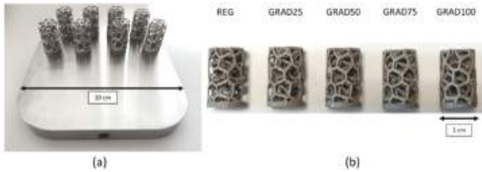
Fig. 2. As-fabricated Ti6Al4V components: example of one of the printed building platform (a); comparison between designed models and fabricated ones (b).
