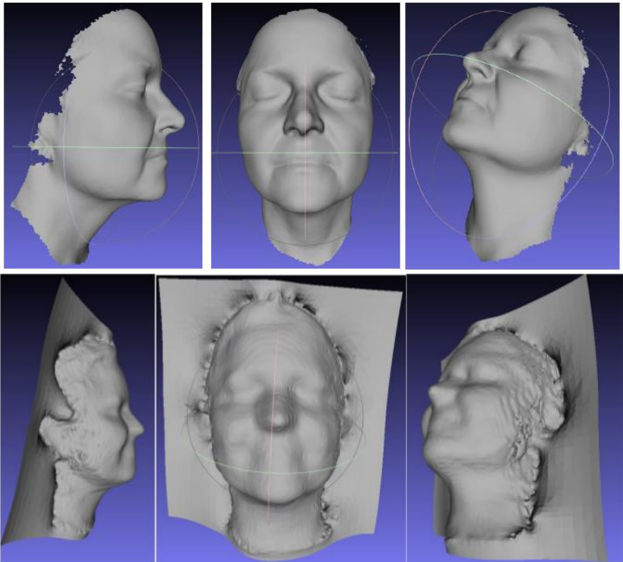
Figure 5. Samples reconstructions from Artec (top panels ) and WM scanner (bottom panels)
