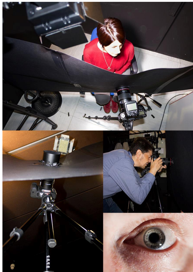
Figure 4. Eye Images acquisition setup with a sample image on the bottom right panel.
