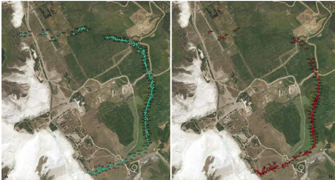
FIG. 11 – Geodatabase of the city walls of Hierapolis showing the location of the travertine (A) and marble (B) architectural elements re-used in the fortifications. The black numbers correspond to the codes used in the geodatabase.
