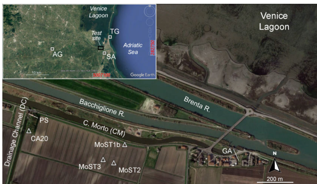
Figure 3. The southern Venice lagoon—coastal area test site with the location of the piezometers (MoST1b, MoST2, MoST3, and CA20), the monitoring points of the surface water levels of the drainage channel (DC) controlled by the pumping station (PS), and the Canal Morto (CM). SA and AG are the locations of meteorological stations, Sant’ Anna and Agna, respectively, while Chioggia tide gauge station is denoted by TG and GA indicates gates at CM.
