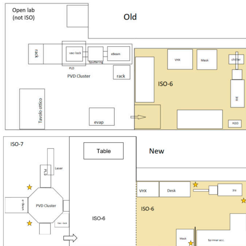
Figure 19. Layout of the production facility. TOP—Old configuration. BOTTOM—New configuration.
