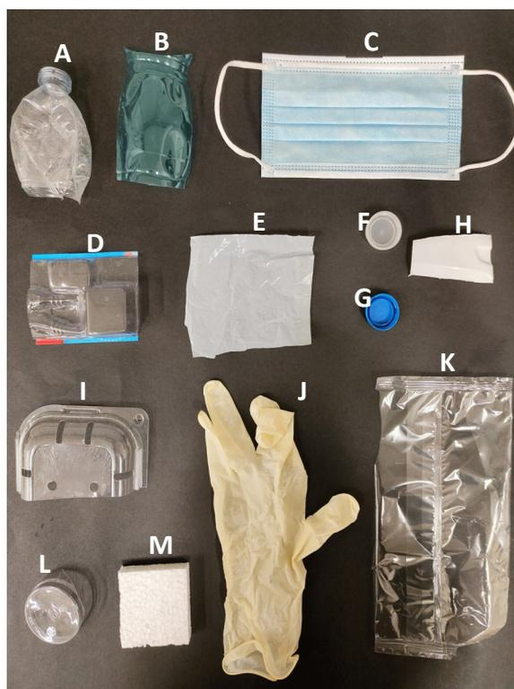
**Figure 1.** Picture of the used commercial plastic samples used in the fluorescence LIDAR experiment. The meaning of the labels (A,B,C,D,E,F,G,H,I,J,K,L,M) is detailed in Table 1.
