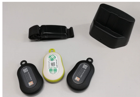
Fig. 2: Social and environmental BLE beacons with the NESTORE wristband and its charging station.
