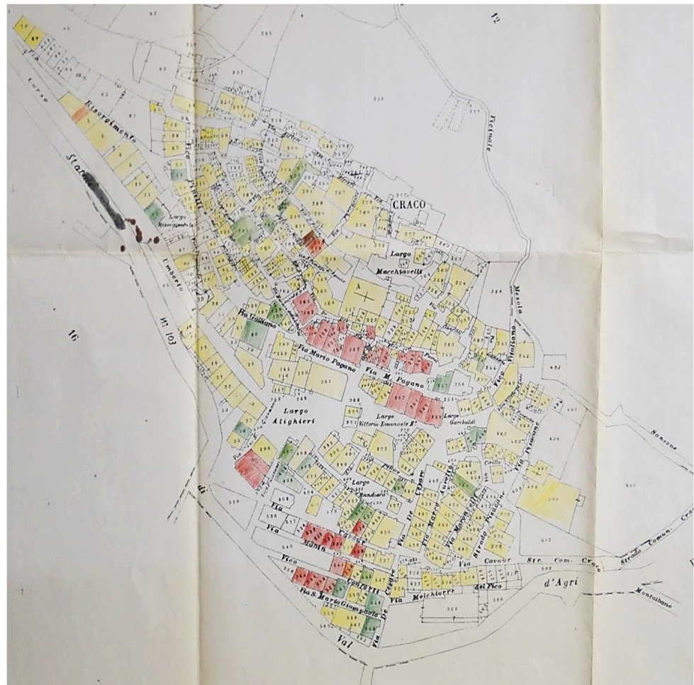
Figure 8. Original map of damage caused by 1963 landslide reactivation in Craco historical center; effects were ascertained with coeval-to-landslide field surveys. Buildings that suffered lesioni forti (heavy cracks) are depicted in red; those that suffered lesioni notevoli (significant cracks), in green; and those that suffered lesioni lievi (slight cracks), in yellow [161]. North is up.
