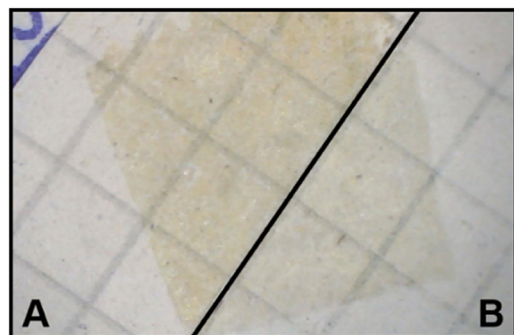
Fig. 8. Images of notebook sample with adhesive tape before (A) and after (B) cleaning with GGMA microgels.
