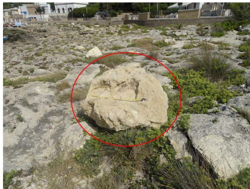
Figure A2. Santa Caterina site; the SCb boulder after the displacement occurred between July 2019 and September 2020 (the image was taken 22 September 2023, with 1 m long tape measure for scale). The whitish surface of SCb is uncovered by lichen and therefore still easily detectable in the field as well as by remote sensing images (see Section 3.1).
