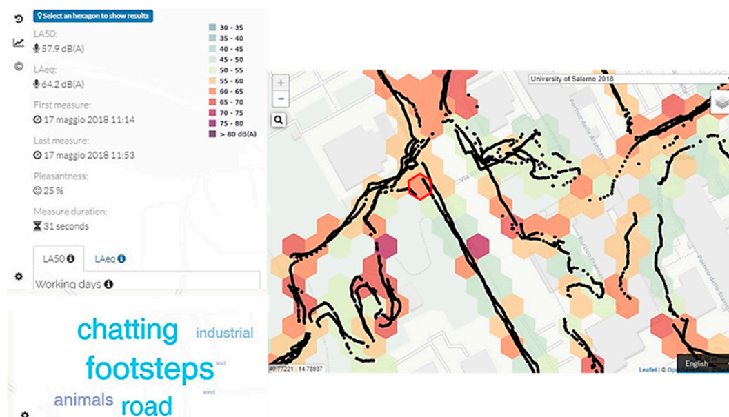
Figure 4. Excerpt of the screenshot of a community noise map available in the Noise-Planet web platform; sound measurements taken at the University campus of Salerno, Italy. Data on the left refer to the hexagon highlighted by red borders.
