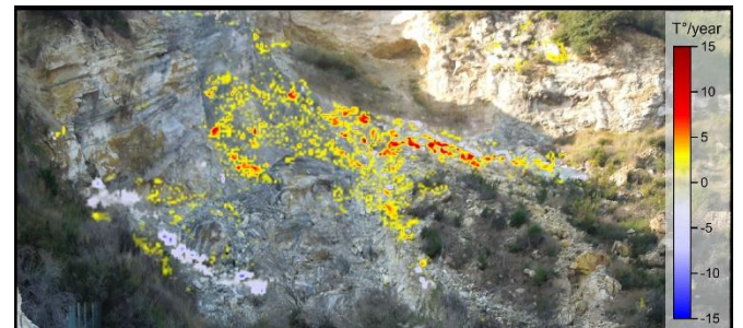
Fig. 5. Map of the temperature rate of change ( dT/yr ) of Pisciarelli investigated area, computed for a period of temperatures increase. The overlapping image masks the values whose R^2 < 0.3 ( R^2 = coefficient of determination).
