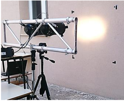
Fig. 2. Outdoor setup of IRT measurements
