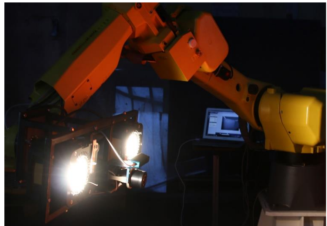
Fig. 23 IR3D Analysis system mounted on robot, performing an automatic inspection of a part of wind-turbine blade from both sides
