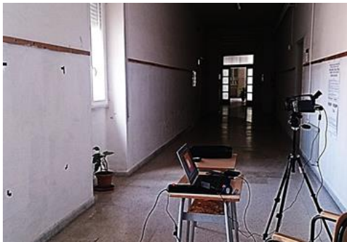
Fig. 3. Inner setup of IRT measurements
