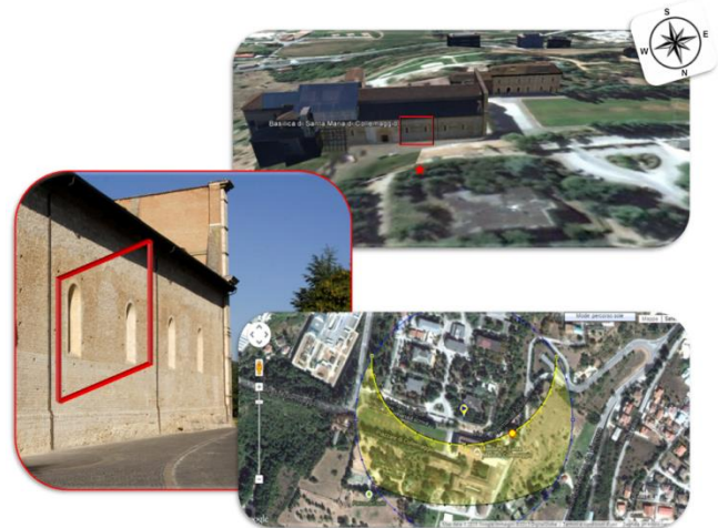
Fig. 2. Thermographic inspection of the lateral Collemaggio façade showing from top to bottom: the position of the infrared camera, the inspected part linked, and the satellite view of the Church showing the sun path during the day of acquisition (June 07 th 2013, image from www.sunearthtools.com ).
