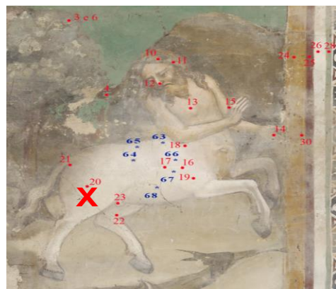
Fig. 4. In situ FORS measurements on selected points of the wall paintings
