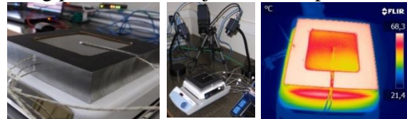
Fig. 1. Photos of the experimental setup for emissivity characterization versus temperature of the composite.
