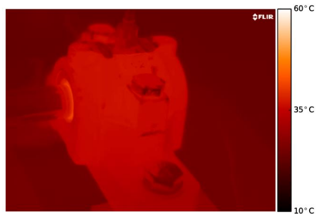
Fig. 17. Example of a thermal image of the bearing housing
