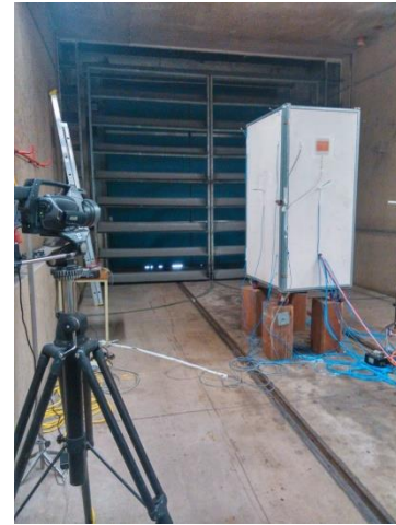
Figure 2: Roll container and equipment utilized for the experimental tests: infrared camera, thermocouples, RTD, and heat flux meter.
