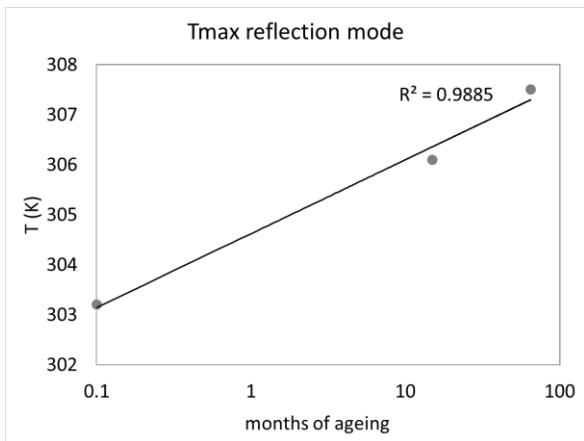
Fig. 3. Logarithmic of the maximum temperature reached after 5 minutes of heating in the reflection mode set up. This fit shows a correlation index of 0.99.
