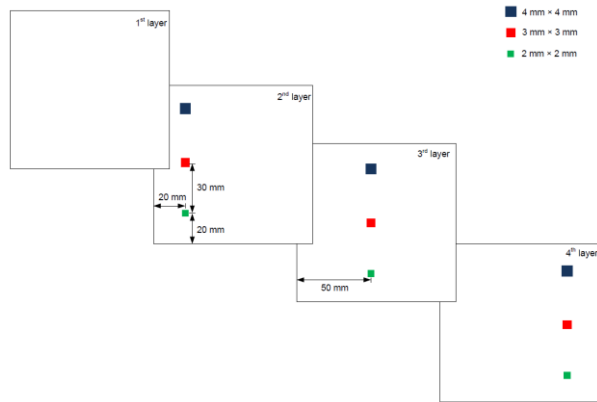
Figure 1 – Position of the artificial inserts on the layers of the laminate
