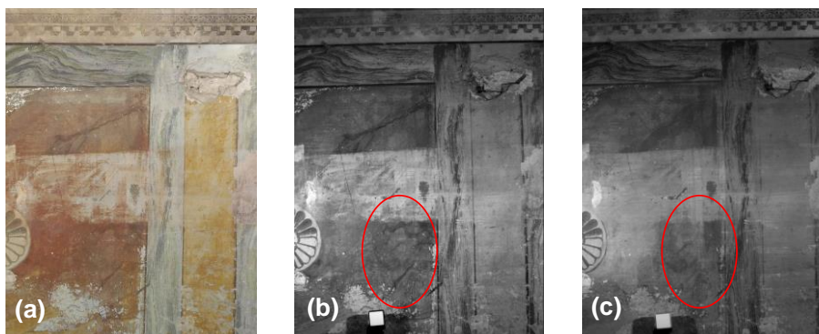
Fig. 3. IR imaging on wall paintings: (a) photo of the investigated area; (b) image acquired in the 600-nm spectral band and (c) image in the 1050-nm band. The area was 90 cm x 115 cm.
