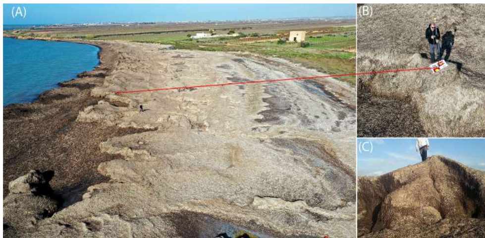
FIGURE 2 | (A) Aerial photograph of the banquette along the coast of Faro beach in the Capo Feto area. (B) Ground control point (GCP) measurement by GNSS receiver. (C) Detail of a banquette Mega-ridge.
