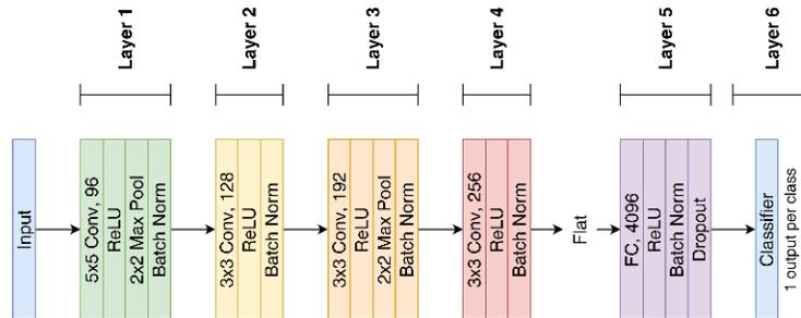
Fig. 3: The neural network used for the experiments.
