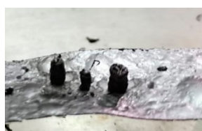
Figure 10. Particle recovered at the end of the naphthalene pitch pyrolysis experiment at a target strip temperature \approx 1600 °C.
