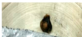
Figure 7. Particle recovered at the end of the cellulose pyrolysis experiment at a target strip temperature of \approx 1000 °C.
