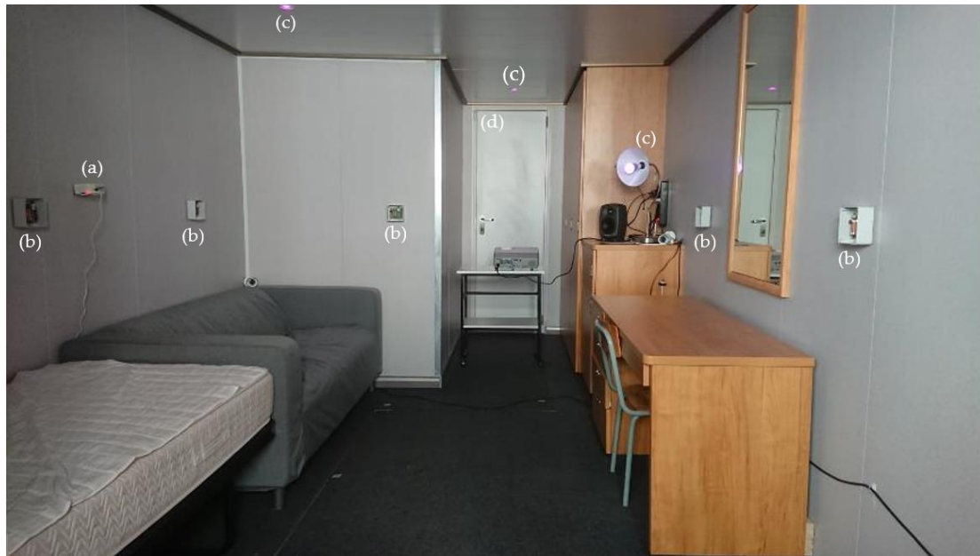
Figure 9. Inside view of the experimental cabin exposing some of the deployed sensors: (a) Noise sensor, (b) indoor localization anchors, (c) controllable light bulbs, and (d) door/movement/light sensor.
