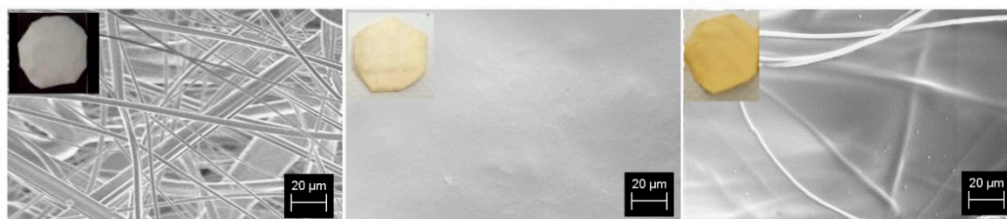
Figure 1. SEM images of PP (left), s-PBC@PP (middle) and s-PBC@PP after UV irradiation (right) samples.
