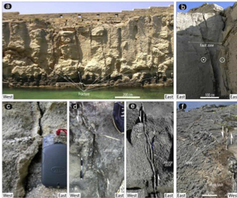
Fig. 4. Examples of brittle structures affecting the Quaternary calcarenite; (a) m-thick spaced, sub-vertical, fractures cemented by calcite; (b) particular of a left-lateral oblique-slip fault zone characterized by anastomosed shear fractures cemented by calcite; (c) detail of the shear fracture cemented by calcite, supporting for infiltration of fluids; (d) extensional jogs filled by calcite in a left-lateral strike-slip fault zone; (e) anastomosed left-lateral strike-slip shear fractures cemented by calcite; (f) Splay system developed within the damage zone of a main left-lateral strike-slip fault.
