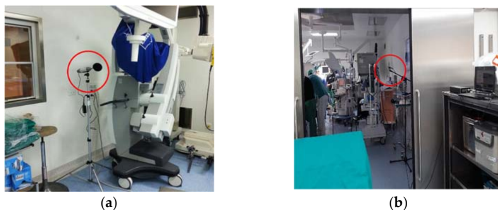
Figure 1. Example of the microphone's location, highlighted by the red circle, selected for the noise measurement in the surgical room: (a) survey 1, (b) survey 2.
