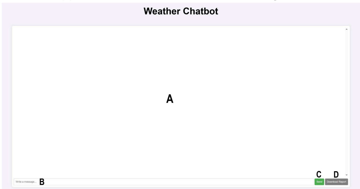
Figure 6. Chatbot’s Interface: in the center is the conversation window (A), where the user can see the sent and received messages. At the bottom, there is a text field that allows the user to type in their questions (B), as well as the “Send” (C) and “Download Report” (D) buttons.
