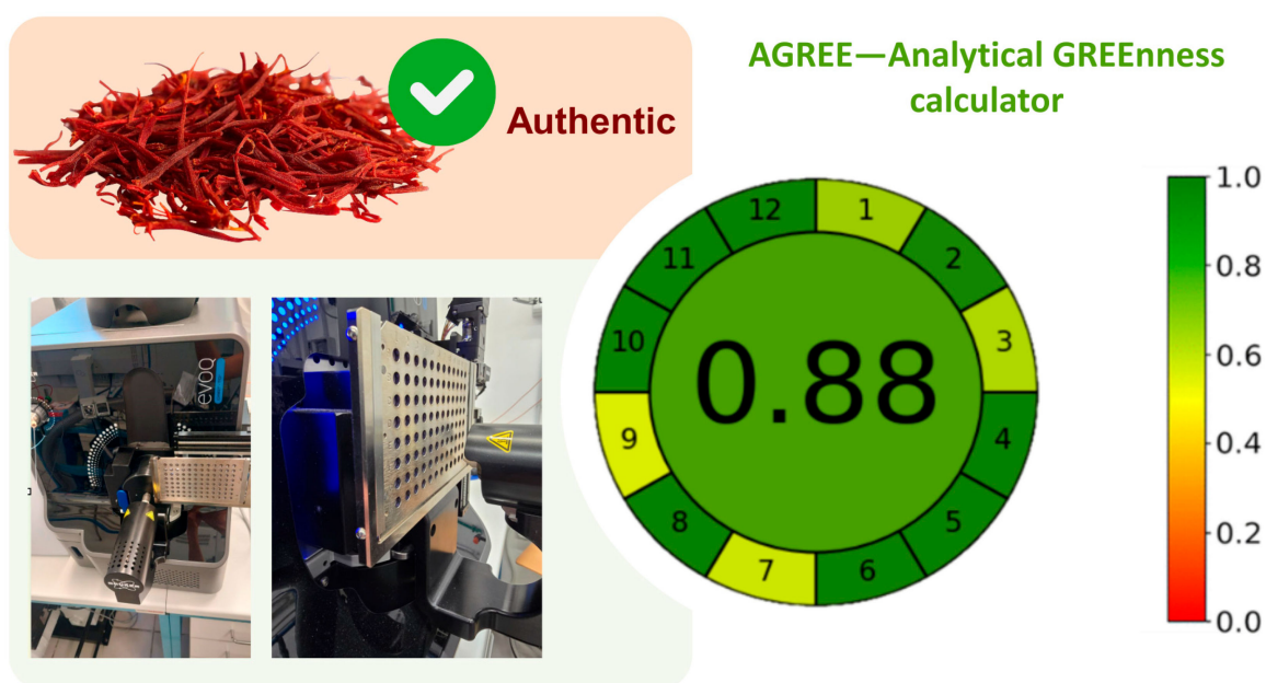
Figure 4. Greenness assessment of the DART-MS/MS method ( left ) and the corresponding colour scale for reference ( right ) by using the AGREE software.
