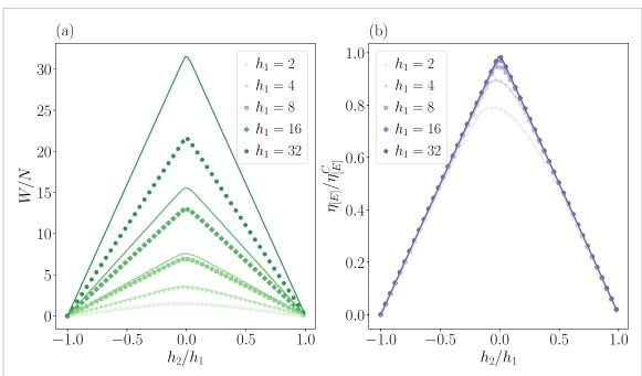
**Figure 4.** Work output (panel (a)) and engine efficiency (panel (b)), plotted as a function of  $h_2/h_1$ , for different values of  $h_1$  corresponding to different colors. Exact values (28c) are represented as scatter plots with different markers (one for each value of  $h_1$ ), while bold lines refer to the approximated result of equation (32). The system size is N = 200, the temperatures of the baths are fixed to  $T_1 = 100$ ,  $T_2 = 0.01$ .
