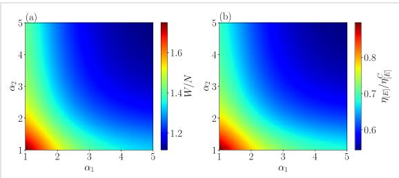
**Figure 12.** Work output (panel (a)) and engine efficiency (panel (b)) plotted as a function of  $\alpha_1$  and  $\alpha_2$ , for fixed values of the cycle parameters in the optimal region:  $h_1 = 2$ ,  $h_2 = 0$ ,  $T_1 = 100$ ,  $T_2 = 0.01$ , and for system size N = 200.
