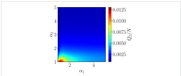
**Figure 14.** Heat exchanged with the cold reservoir plotted as a function of  $\alpha_1$  and  $\alpha_2$ , for cycle parameters:  $h_1 = 2$ ,  $h_2 = -1 + 2^{1-\alpha_1}$ ,  $T_1 = 0.1$ ,  $T_2 \simeq 0.099$ , and for system size N = 200.
