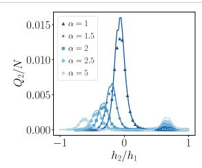
**Figure 7.** Heat extracted from the cold reservoir  $Q_2$ , as a function of  $h_2/h_1$ . Scatter plots indicate the exact values (28b), bold lines indicate the approximated result (35). Different colors correspond to different values of  $\alpha_1 = \alpha_2 = \alpha$ . The baths temperatures are fixed to  $T_1 = 0.1$ ,  $T_2 \simeq 0.099$ .
