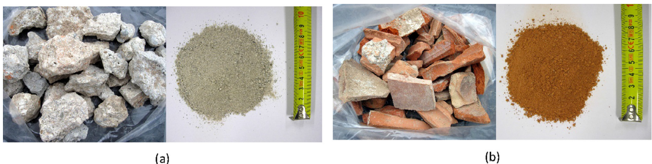
Fig. 1. Waste before and after milling: (a) concrete CR1, and (b) fired clay FC1.
