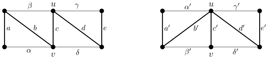
Figure 2: Two 2-isomorphic graphs that are not isomorphic: x \mapsto x' maps bijectively fundamental cycles of the graph on the left to fundamental cycles of the graph on the right.
