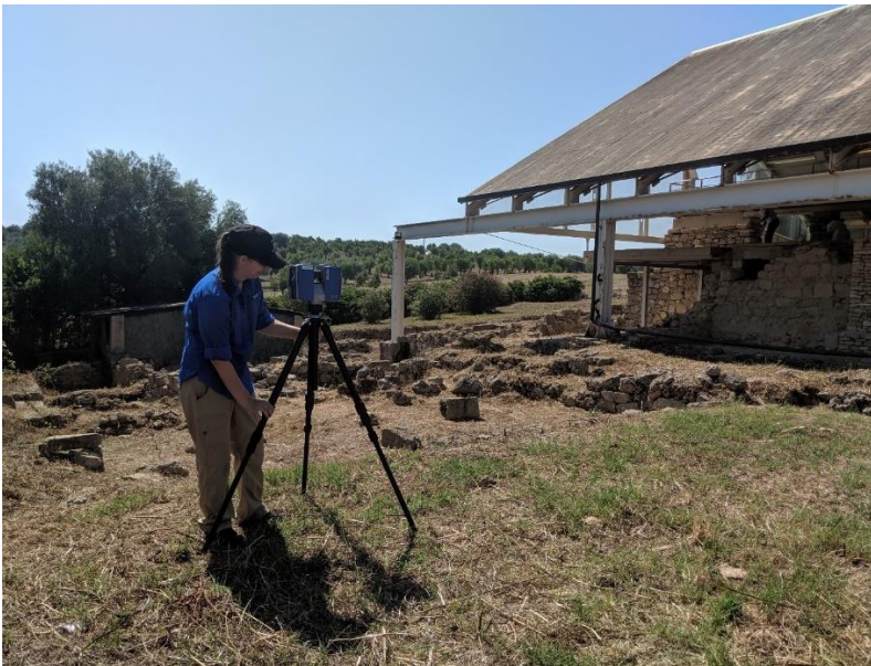
Figure 2. Terrestrial laserscanning at the Villa employing a Faro Focus x330.
