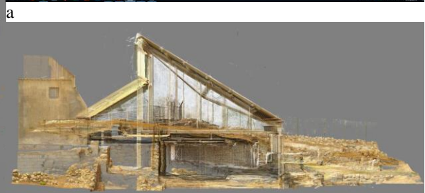
Figure 5. a) 3D point cloud model processed with Faro Scene 2019.a; b) north-south section view of the point cloud model of the villa.
