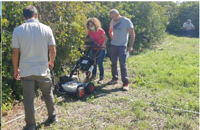
Figure 15. GPR survey in Area 2.
