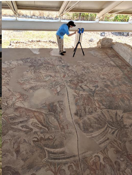
Figure 3. Terrestrial laserscanning of the room of the Hunt mosaic
