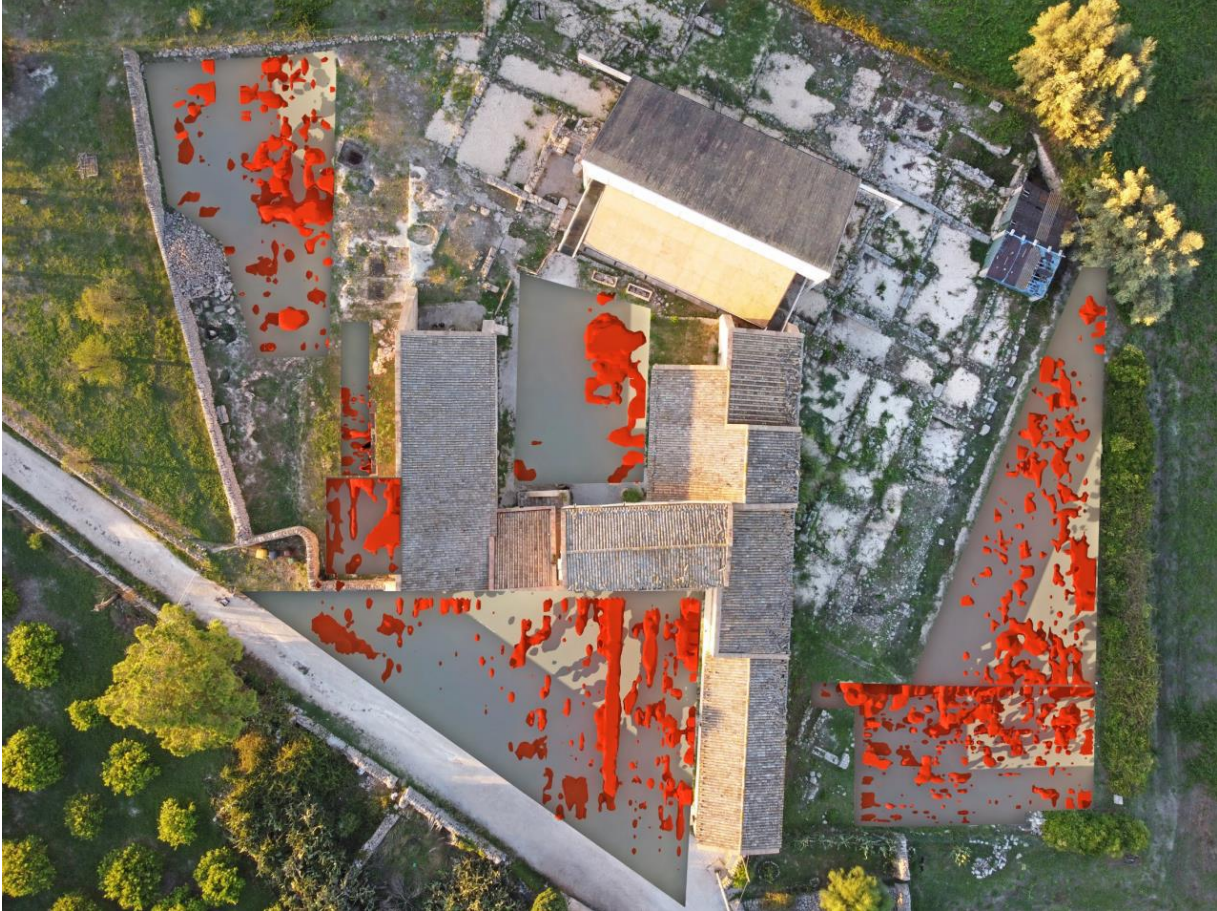
Figure 42. Superimposition of iso-surface amplitudes of all areas onto aerial photograph, creating a 3D representation of the anomalies detected in context.
